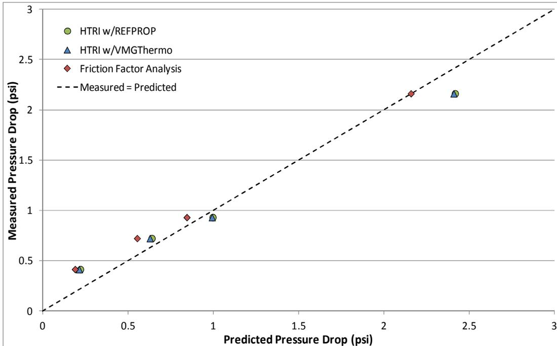
**Figure 3. S-CO<sub>2</sub> Tube Side Pressure Drop in the IHX.**
