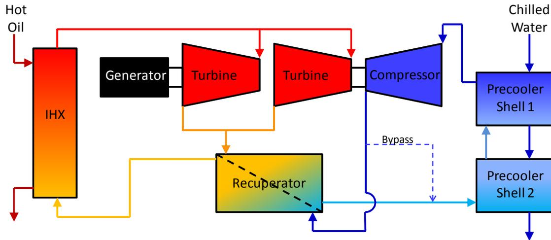
**Figure 1. Schematic of the IST S-CO<sub>2</sub> Brayton Test Loop.**
