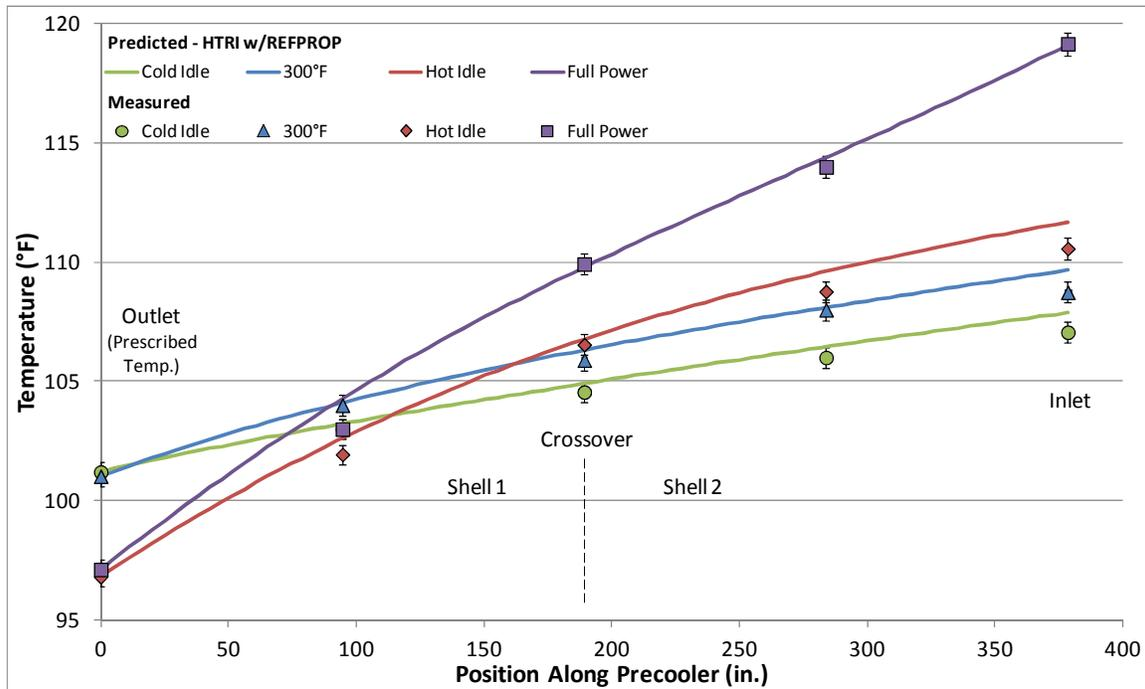
**Figure 5. Precooler Shell-side S-CO<sub>2</sub> Temperature Profiles**
