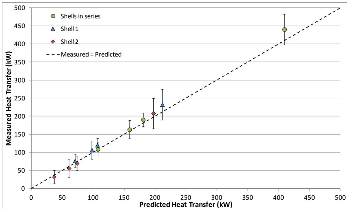
**Figure 4. Comparison of Measured Heat Transfer Rates to HTRI Model Prediction for the Shell Side (S-CO<sub>2</sub>) of the IST Precooler.**
