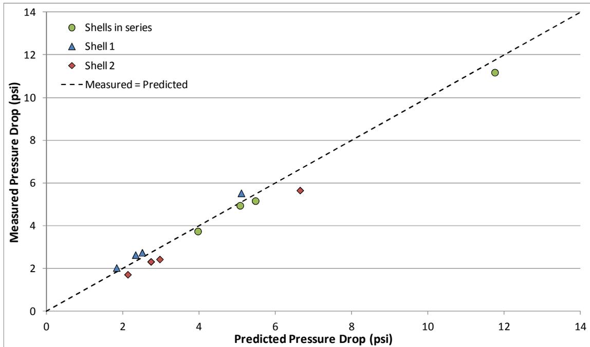
Figure 6. Pressure Drop in the IST Precooler Shell.
