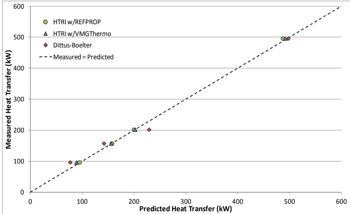
**Figure 2. Measured versus Predicted Tube Side S-CO<sub>2</sub> Heat Transfer Rates for the IHX.**
