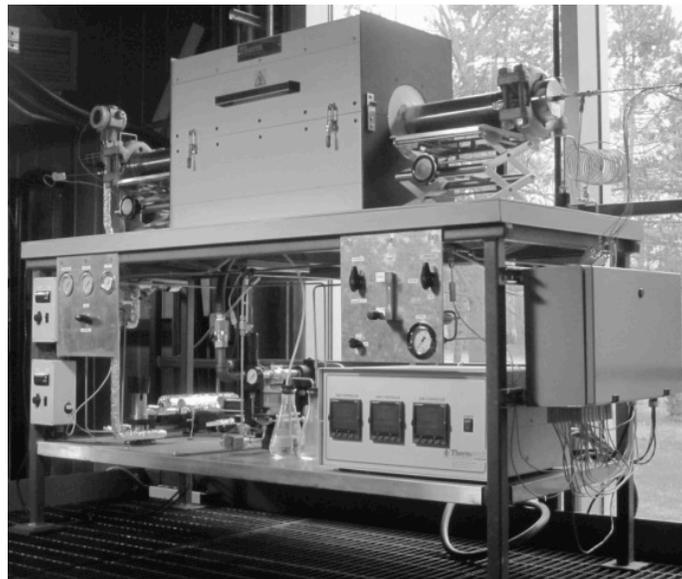
**Figure 2: NRCan-Carleton University corrosion test rig.**
