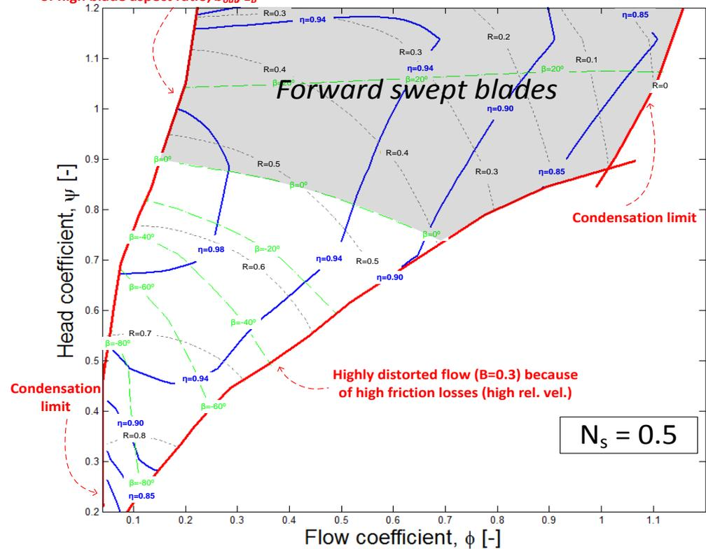
$$\phi = \frac{v_{x1}}{u_2} \quad \psi = \frac{\Delta h_{0s}}{u_2^2} \quad R = \frac{h_2 - h_1}{\Delta h_0} \quad N_s = \frac{\omega \sqrt{Q}}{\Delta h_s^{3/4}}$$
