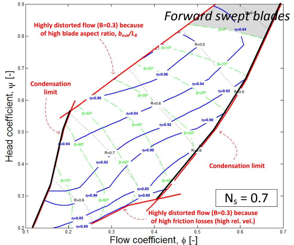
$$\phi = \frac{v_{x1}}{u_2} \quad \psi = \frac{\Delta h_{0s}}{u_2^2} \quad R = \frac{h_2 - h_1}{\Delta h_0} \quad N_s = \frac{\omega \sqrt{Q}}{\Delta h_s^{3/4}}$$
