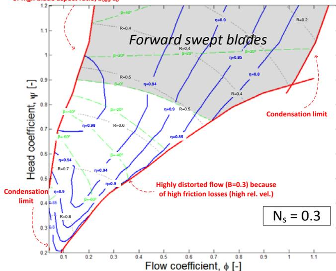
Highly distorted flow ( $B=0.3$ ) because of high blade aspect ratio,  $b_{out}/L_B$
