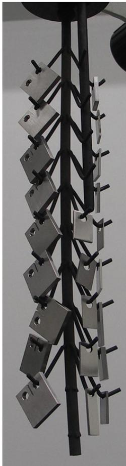
Fig. 2. Sample rack and samples for  $sH_2O$  exposure in a vertical autoclave. Rack hooks were made from alloy 617.
