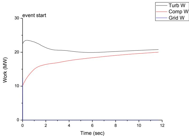
**Figure 10. Work of turbomachinery on load rejection without active control**
