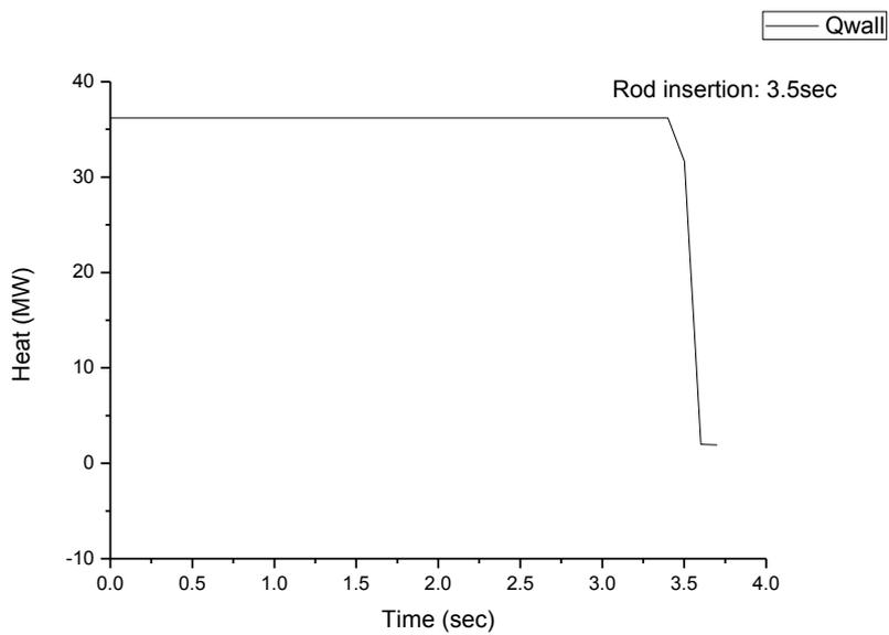
**Figure 14. Reactor trip by rod insertion**
