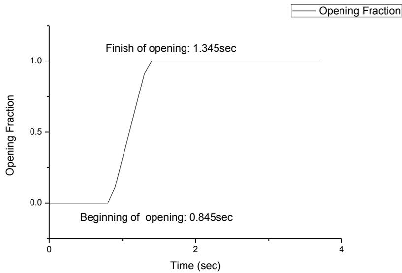
**Figure 13. Core inlet bypass valve opening rate**
