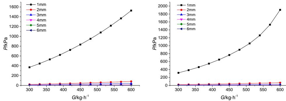
Figure.12. Channel Width Influence on PCHE Pressure Drop
