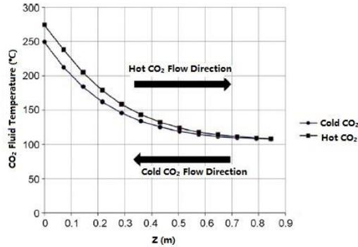
Figure.6. Kim Simulation of Cold and Hot Fluid Temperature Change along the Wall
