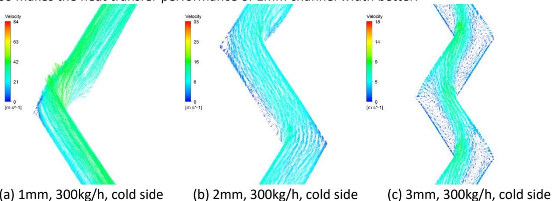
Figure.13. Velocity Vector Distribution of the Typical Channel Width
