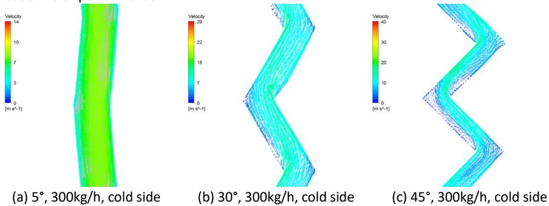
Figure.17. Velocity Vector Distribution of the Typical Fin Angle
