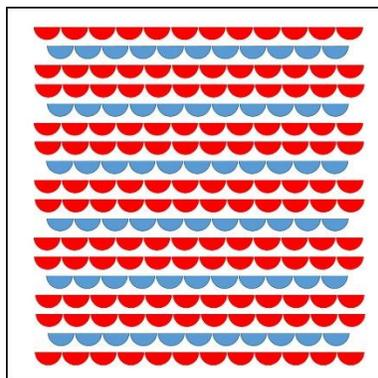
Figure.3. PCHE Cold and Hot Channels Arrangement
