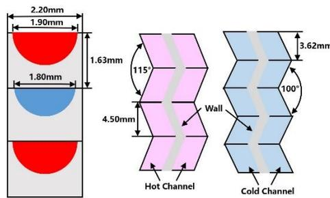
Figure.4. PCHE Channel Unit Structure Parameters
