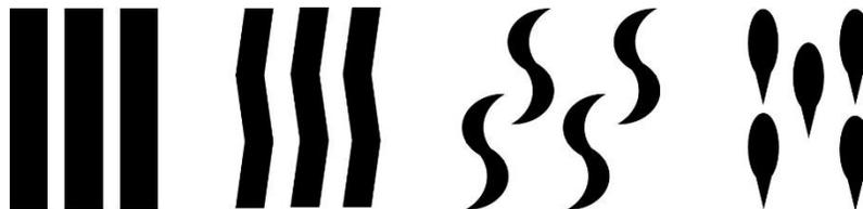
Figure.2. Different PCHE Flow Channels
