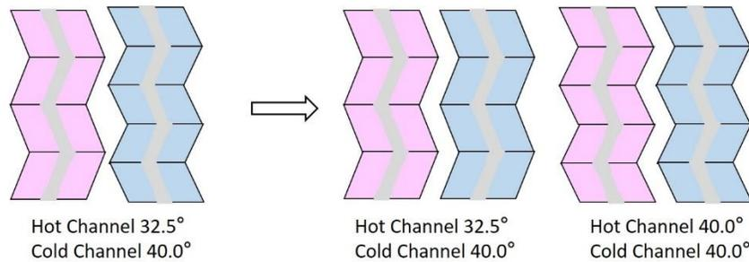
Figure.5. Experiment Model Simplification
