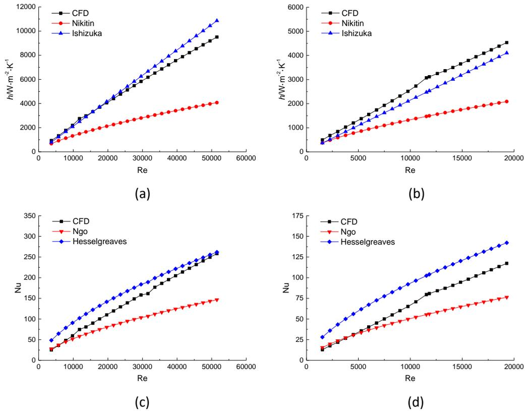
Figure.8. Heat Transfer Performance at Fin Angle 32.5° in Cold and Hot Side
