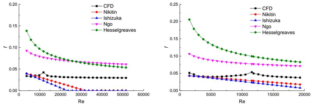
Figure.9. Pressure Drop at Fin Angle 32.5° in Cold and Hot Side
