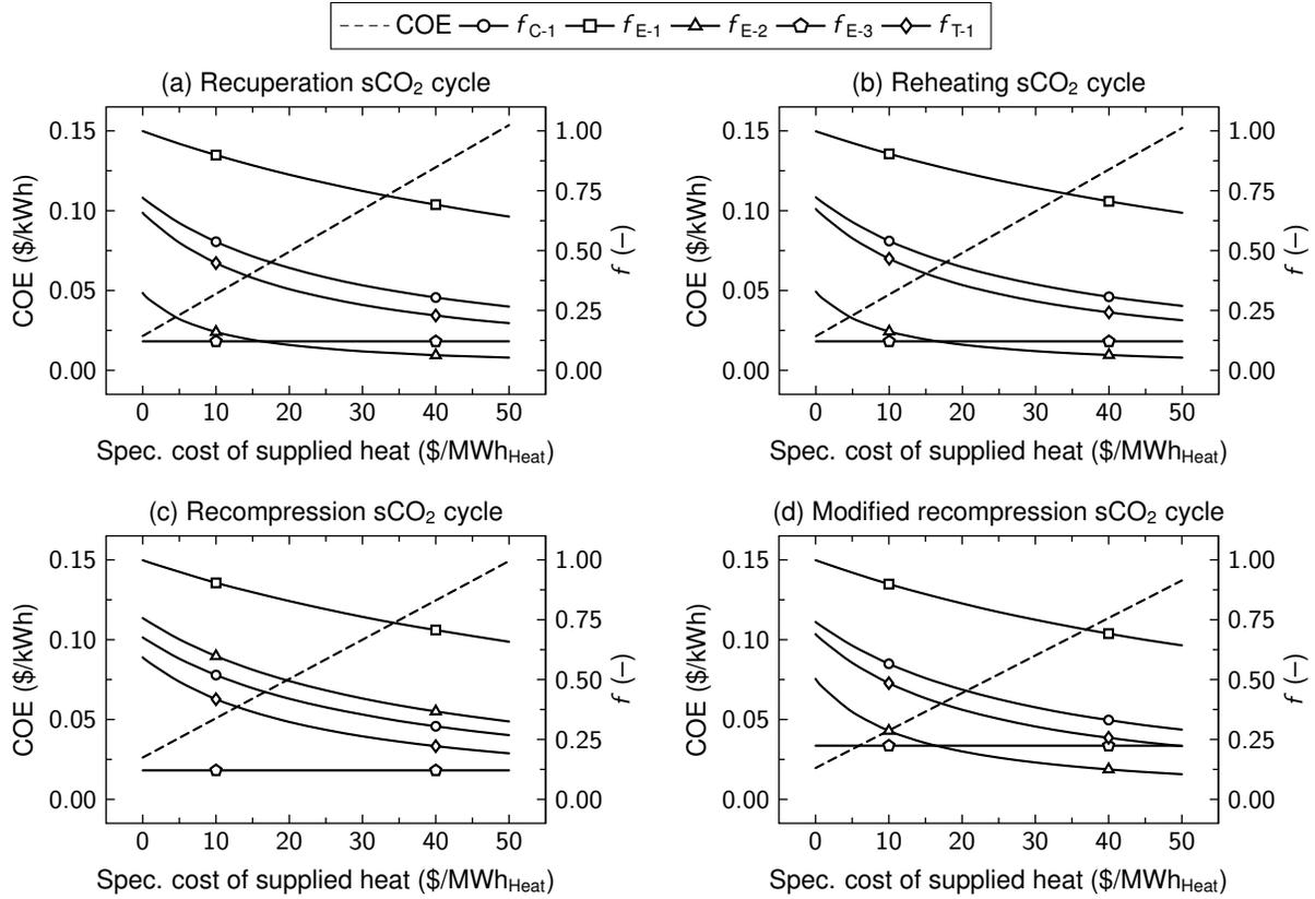
Figure 2: Sensitivity analyses of the simple sCO<sub>2</sub> cycle configurations regarding the influence of the cost of supplied heat.
