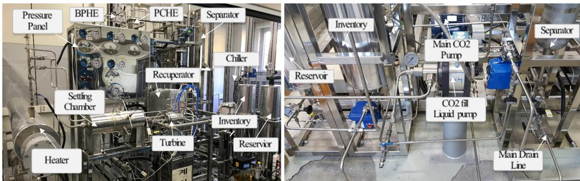
Figure 7. A tens of kWe-class transcritical supercritical CO<sub>2</sub> power cycle test loop
