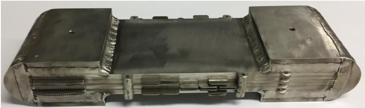
**Fig. 23.** PCHE with reinforced header region
