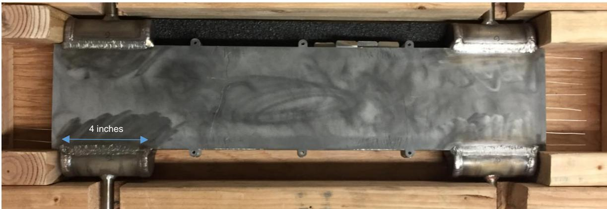
**Fig. 5.** Prototypic PCHE with internal capillary tubes (seen on right end).
