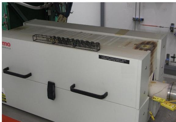
Figure 2. Rack of test coupons resting on top of one of the tube furnaces prior to reloading for additional exposure testing.
