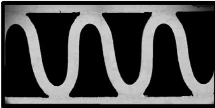
347H, 5000h at 700°C in sCO<sub>2</sub> - 3.6% O<sub>2</sub>-5.3% H<sub>2</sub>O at 200 bar
