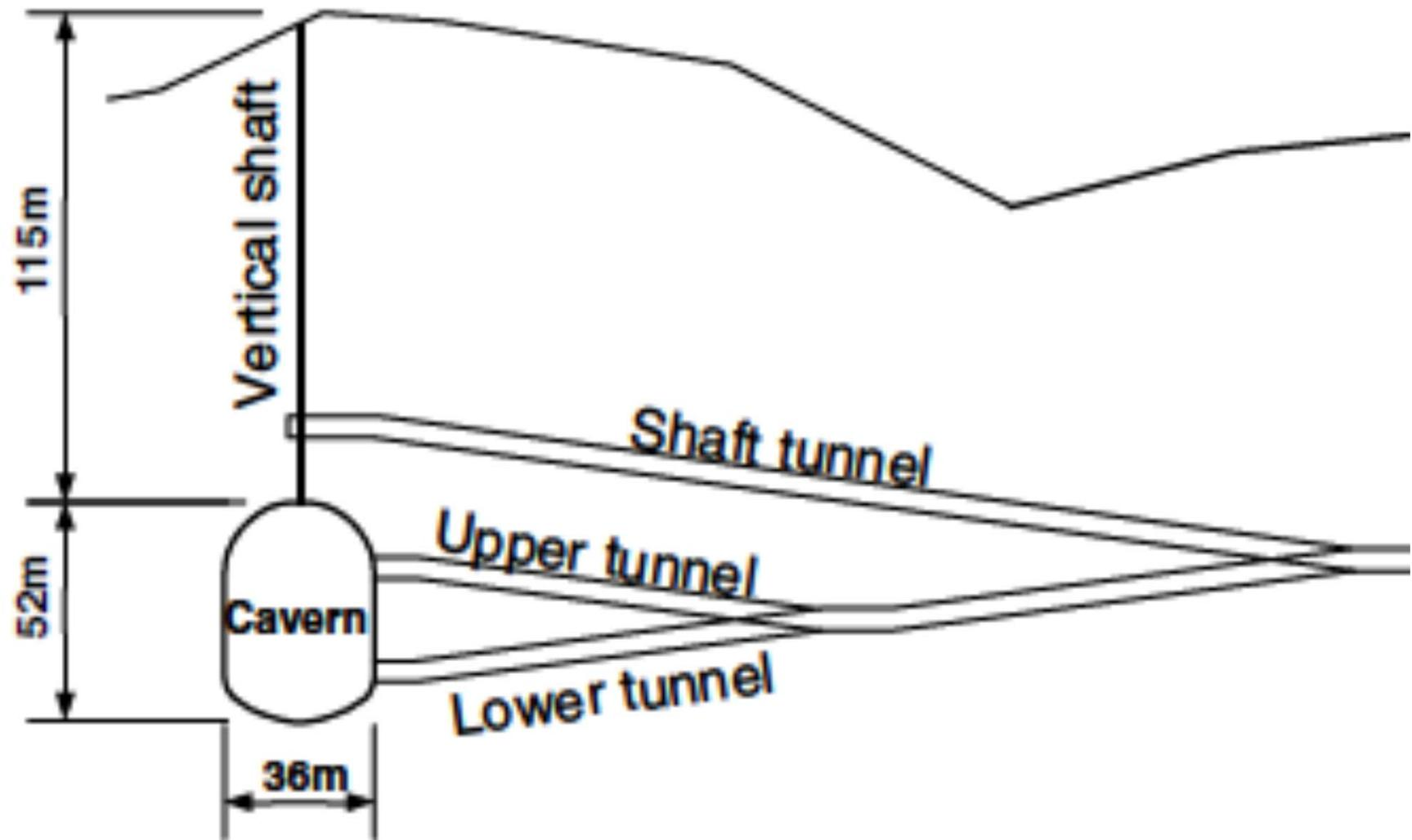
Glamheden, "Excavation of a cavern for high-pressure storage of natural gas", Tunneling & Underground Space Tech., 2006.
